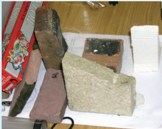
Stone and brick samples for testing of moisture properties by X-ray method at Glasgow Caledonian University
